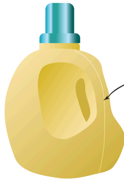
PARTING LINES ON INJECTION MOLDED PLASTICS
