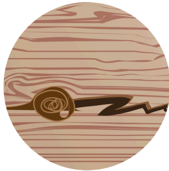
LOOSE KNOTS AND CRACKS IN WOOD
