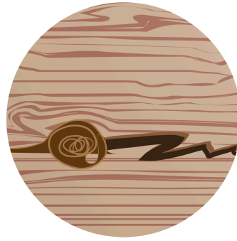
LOOSE KNOTS AND CRACKS IN WOOD
