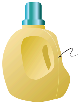
PARTING LINES ON INJECTION MOLDED PLASTICS
