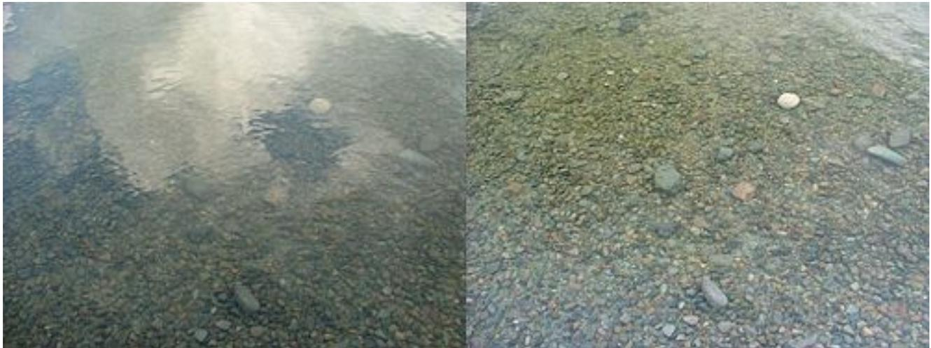
Figure 11: An example of looking at shallow water, without (left) or with (right) a polarization filter. Reflection Polarizer2, by Amithshs, Wikimedia Commons, public domain.
