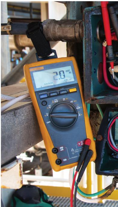
When handling a multimeter it is wise to be sure the meter is held securely. Dropping a multimeter, especially an analog meter, even from a small height can affect future readings and the accuracy of the multimeter. While taking readings the user is most likely going to need the use of both hands to complete the task. As a result it is
