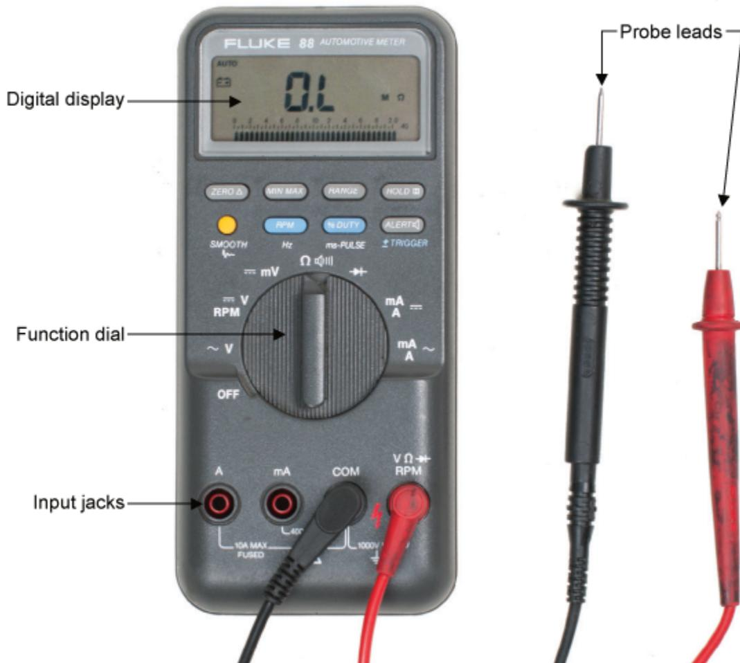
The upper portion of the DMM houses the display unit. The middle portion of the DMM houses the function switch, and the bottom portion contains the jacks for test leads.
