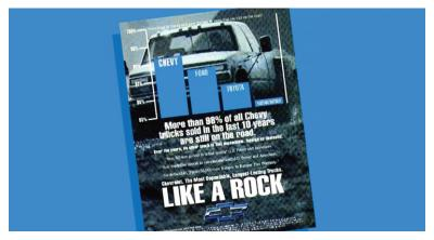
And this is how they presented this data; From this graph, it seems like Chevy trucks are almost two times more reliable than Toyota and ten times more reliable than Nisssan/Datsun. However, when we look at the y-axis, we realize the scale range is from 95% to 100%; so a seemingly big difference is actually nothing at all.
