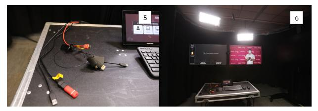
Photo 5 includes a user laptop connection (HDMI), available adapters, a USB connection for connecting to the presentation clicker available (optional) and USB input for recording media
