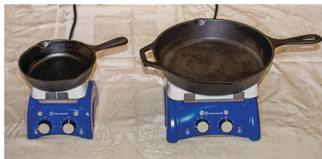
Figure 4.2g: Due to its larger mass, a large frying pan has a larger heat capacity than a small frying pan. Because they are made of the same material, both frying pans have the same specific heat. (credit: Mark Blaser in Chemistry (OpenStax) , CC BY 4.0).
