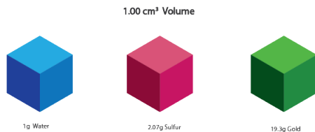
Figure 2.1d: The figure shows 3 cubes. Each of equal volume but with varying masses. (credit: graphics by Revathi Mahadevan, CC BY 4.0)
