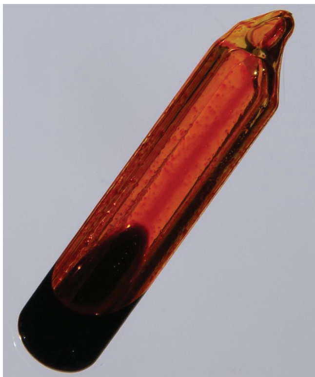
Figure 17.2d: An equilibrium is pictured between liquid bromine, \text{Br}_2(l) , the dark liquid, and bromine vapour, \text{Br}_2(g) , the orange gas. Because the container is sealed, bromine vapour cannot escape and equilibrium is maintained. (credit: work by Anonymous/Images of Elements, CC BY 3.0 )
