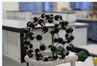
Figure 11.3t: This model shows the arrangement of carbon atoms in a fullerene (or ‘buckyball’) a large molecule made up of 60 carbon atoms. (credit: work by UCL Mathematical and Physical Science ( https://www.flickr.com/people/93636241@N07 ), CC BY 2.0)
