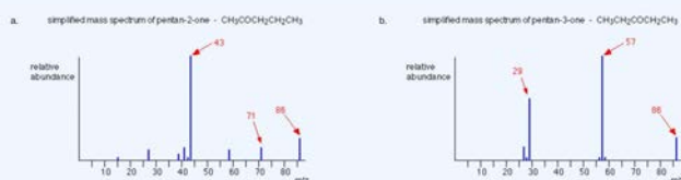
Figure 29.7e. a) Mass spectrum of pentan-2-one and b) Mass spectrum of pentan-3-one (credit: Map: Organic Chemistry (Wade) , CC BY-NC-SA 4.0).
