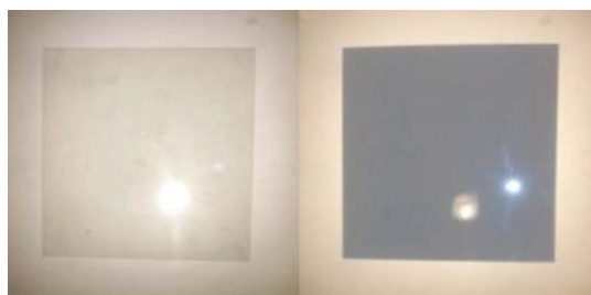
Figure 28.1f. In the photo on the left, two Polaroid sheets are aligned in the same direction; plane-polarized light from the first Polaroid sheet can pass through the second sheet. In the photo on the right, the top Polaroid sheet has been rotated 90^\circ and now blocks the plane-polarized light that comes through the first Polaroid sheet (credit: Intro Chem: GOB (V. 1.0) , CC BY-NC-SA 3.0).
