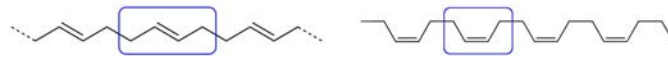
Figure 27.5d. Trans (left) and cis (right) -1,4-polybutadiene (credit Images a & b by Jü; CC0)
