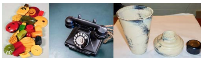
Figure 27.1f. Examples of products made from Bakelite (credit a: “Set of Phenol formaldehyde resin buttons” by Gregory Tobias, CC BY-SA 3.0; b: work by William Warby ( https://www.flickr.com/people/26782864@N00 ), CC BY 2.0; c: work by Tangerineduel, CC BY-SA 4.0).
