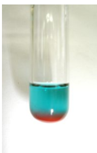
Figure 24.4g. Oxidation of aldehyde with Benedict's reagent. Original blue reagent on top and resulting red precipitate on bottom. This is a positive result (credit: Image by Kala Nag, CC BY-SA 4.0).
