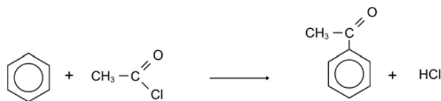
Figure 22.5u. Benzene reacts with \text{CH}_3\text{COCl} and aluminum chloride as the catalyst to produce phenylethanone. (credit: Supplemental Modules (Organic Chemistry) , CC BY-NC 4.0).
