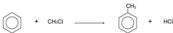
Figure 22.5w. The reaction of chloromethane with benzene and aluminum chloride as the catalyst to produce an alkylated benzene.(credit: Supplemental Modules (Organic Chemistry) , CC BY-NC 4.0).
