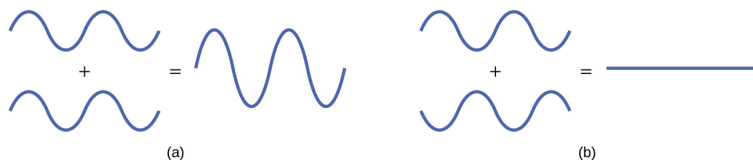
Figure 2. (a) When in-phase waves combine, constructive interference produces a wave with greater amplitude. (b) When out-of-phase waves combine, destructive interference produces a wave with less (or no) amplitude.
