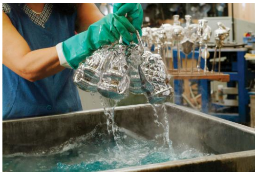
Figure 15.3.1: Aldehyde Reactions. A reaction related to the Tollens' reaction is often used to silver mirrors. These ornaments were silvered by such a reaction. Glucose, a simple sugar with an aldehyde functional group, is used as the reducing agent. Source: Photo courtesy of Krebs Glas Lauscha, commons.wikimedia.org/wiki/File:Silvering.jpg.
