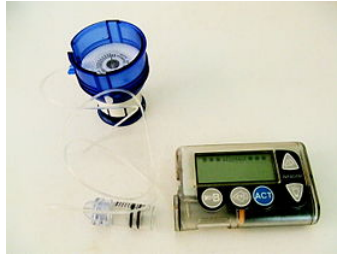
Figure 18.0.1: Insulin pump, showing an infusion set loaded into spring-loaded insertion device. A reservoir is attached to the infusion set (shown here removed from the pump). (Public Domain; User:David-i98 ).
