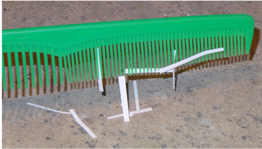
Figure 5.2b Electric Charge Real Life Example 2: After being used to comb hair, this comb attracts small strips of paper from a distance, without physical contact. Investigation of this behaviour helped lead to the concept of the electric force (credit: Jane Whitney in University Physics Volume 2 (Open Stax) , CC BY 4.0).
