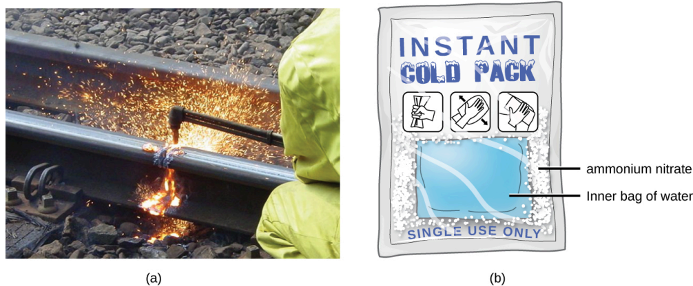
Figure 4.2f (a) An oxyacetylene torch produces heat by the combustion of acetylene in oxygen. The energy released by this exothermic reaction heats and then melts the metal being cut. The sparks are tiny bits of molten metal flying away. (b) A cold pack uses an endothermic process to create the sensation of cold. (credit a: modification of work by Skatebiker, PD; credit b: Chemistry (OpenStax) , CC BY 4.0).
