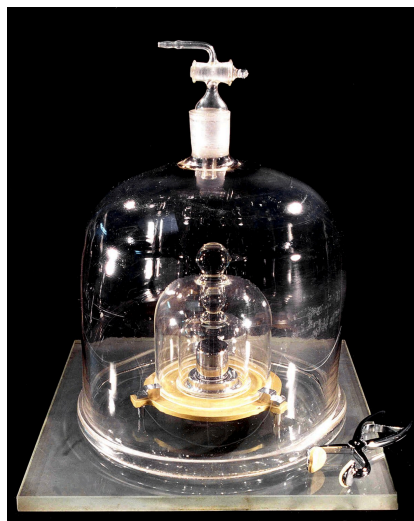
Figure 2.1b This replica prototype kilogram is housed at the National Institute of Standards and Technology (NIST) in Maryland. (credit: photo by BIPM, CC BY-SA 3.0)
