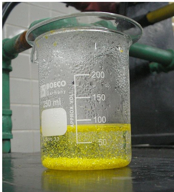
Figure 15.3a Formation of Precipitate Lead(II) Iodide during a Precipitation Reaction: The precipitation reaction producing Lead(II) iodide is shown. It is known as “golden rain” because of the yellow hexagonal crystals forming throughout in the aqueous solution and the solid crystals settle at the bottom of the beaker. This picture was taken after cooling a heated lead(II) nitrate and potassium iodide solution on a Bunsen burner. (credit: work by Der Kreole, CC BY-SA 3.0)
