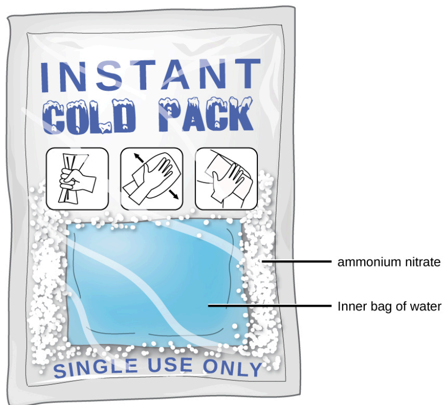
Figure 14.1e An instant cold pack gets cold when certain salts, such as ammonium nitrate, dissolve in water—an endothermic process (credit: Chemistry (OpenStax) , CC BY 4.0).
