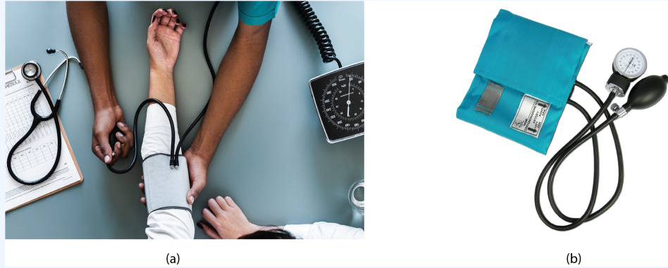
Figure 12.1f (a) A medical technician prepares to measure a patient's blood pressure with a sphygmomanometer. (b) A typical sphygmomanometer uses a valved rubber bulb to inflate the cuff and a diaphragm gauge to measure pressure. (credit a: work by rawpixel.com, CC0; credit b: work by Medisave UK, CC BY 2.0)
