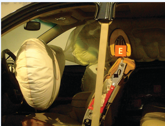
Figure 9.2b Airbags deploy upon impact to minimize serious injuries to passengers. (credit: work by Jon Seidman, CC BY 2.0)
