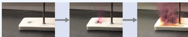
Figure 9.1a Aluminum and iodine react to produce aluminum iodide. The heat of the reaction vaporizes some of the solid iodine as a purple vapour. (credit: modification of work by Mark Ott in Chemistry (OpenStax) , CC BY 4.0).
