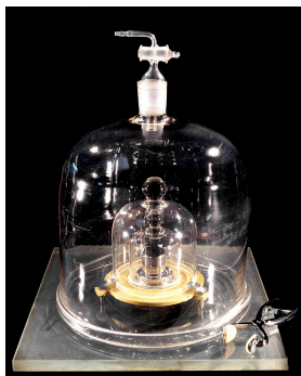
Figure 2.1b This replica prototype kilogram is housed at the National Institute of Standards and Technology (NIST) in Maryland. (credit: photo by BIPM, CC BY-SA 3.0)
