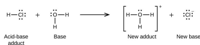
Figure 16.1h Lewis Acid-Base Displacement Reaction: In this reaction, HCl is an acid-base adduct that reacts with water, which is behaving as a base, to form a new adduct (hydronium ion) and a new base (chloride ion) (credit: Chemistry (OpenStax) , CC BY 4.0)
