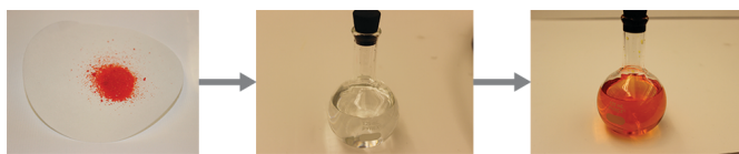
Figure 14.1a When potassium dichromate ( K_2Cr_2O_7 ) is mixed with water, it forms a homogeneous orange solution. (credit: modification of work by Mark Ott in Chemistry (OpenStax) , CC BY 4.0).
