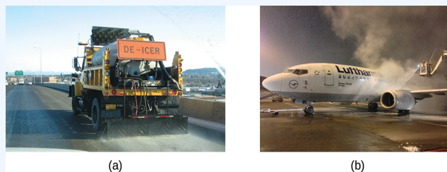
Figure 14.5e Freezing point depression is exploited to remove ice from (a) roadways and (b) the control surfaces of aircraft. (credit a: work by Oregon Department of Transportation, CC BY 2.0; credit b: work by Paolo Cerutti ( https://www.flickr.com/people/76926545@N05 ), CC BY 2.0)
