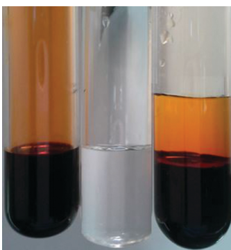
Figure 14.2g Bromine (the deep orange liquid on the left) and water (the clear liquid in the middle) are partially miscible. The top layer in the mixture on the right is a saturated solution of bromine in water; the bottom layer is a saturated solution of water in bromine. (credit: Paul Flowers in Chemistry (OpenStax) , CC BY 4.0).
