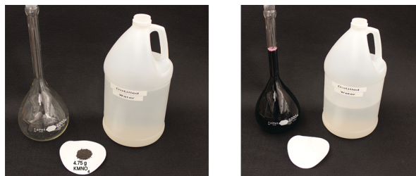
Figure 14.3d A solution of \text{KMnO}_4 is prepared by mixing water with 4.74 g of \text{KMnO}_4 in a flask. (credit: modification of work by Mark Ott in Chemistry (OpenStax) , CC BY 4.0).
