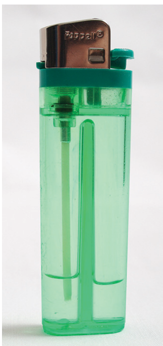
Figure 13.1c Gaseous butane is compressed within the storage compartment of a disposable lighter, resulting in its condensation to the liquid state. (credit: modification of work by Sam-Cat, CC BY 2.0)
